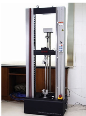
Peeling Strength Test
